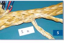
THIS PROCEDURE DESCRIBES THE SPLICE BEING TUCKED 10 1/2 TIMES
